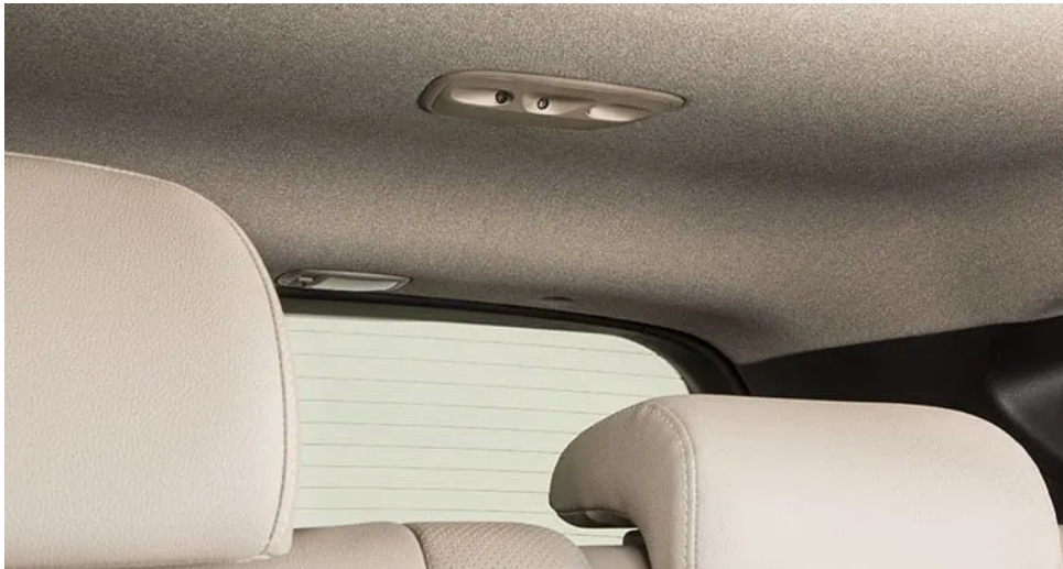
Figure 14: Santa Fe's ultrasonic sensor in the headliner
